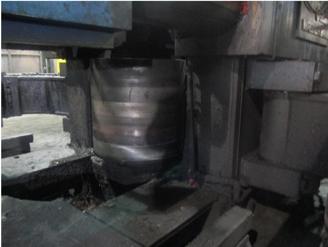
Figure 4 - Machine with automatic cooling water distributor, sump located under machine
