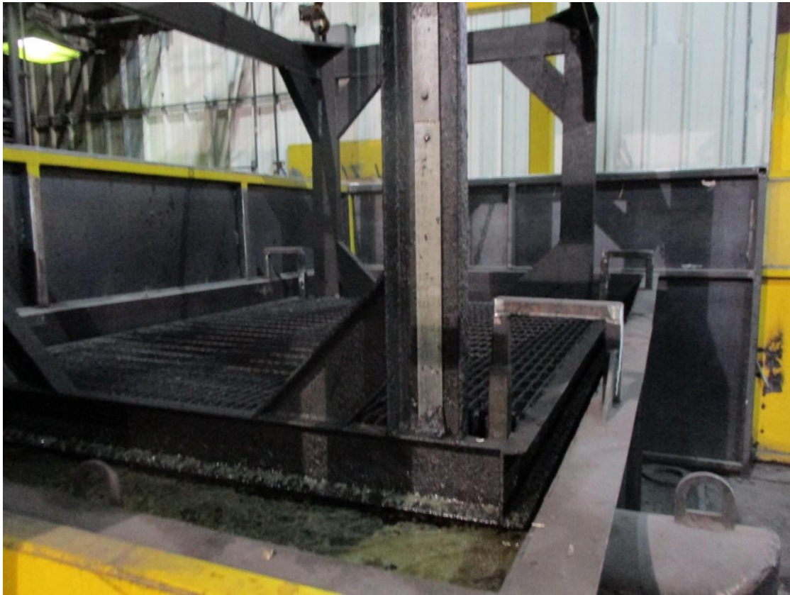
Figure 6 - Small quench tank that utilizes recycled cooling water
