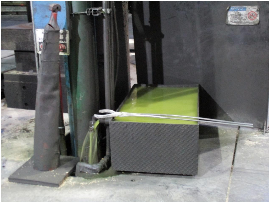
Figure 7 - Small dip tank that uses recycled cooling water
